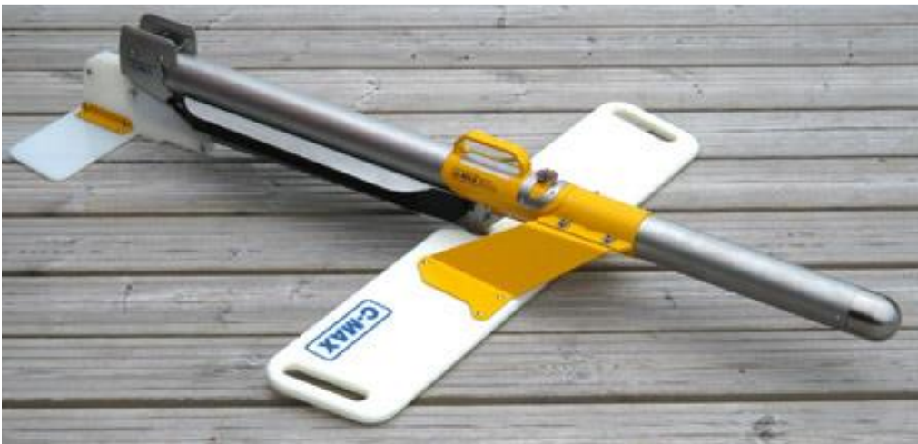
Figure 2. C-MAX CM2 side-scan sonar towfish.
