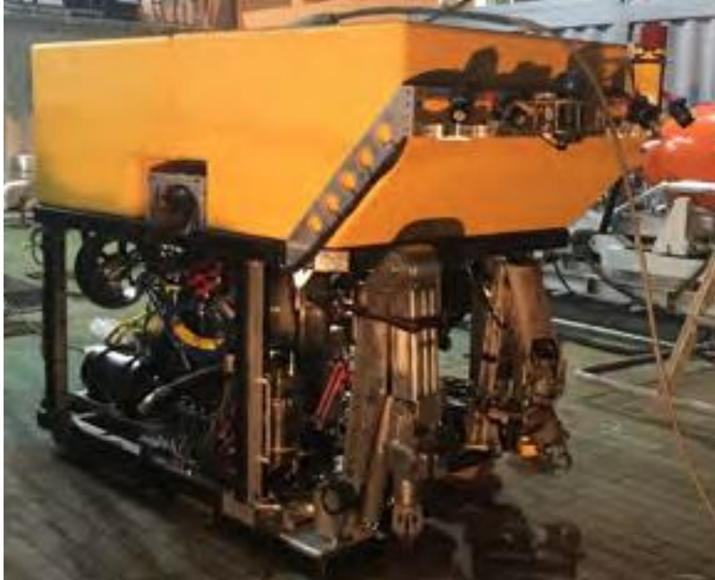
Figure 17. GP-50 remotely operated vehicle (provided by EGI)
